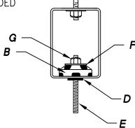
3. SECURE LOWER END OF THREADED ROD (E) TO UNIT BEING SUPPORTED. TAKE CARE THAT THREADED ROD IS CENTERED IN THE HANGER BOX BOTTOM HOLE.
